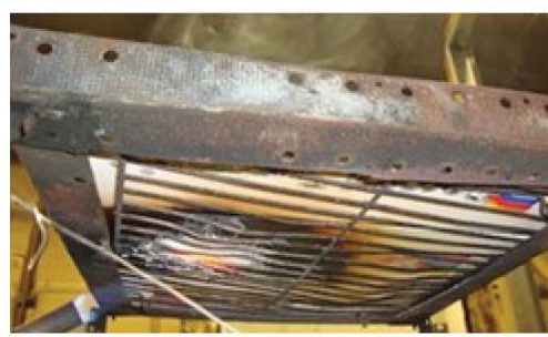
3:00 to 9:00 : No flame spread; light smoke; white intumescence @ torch area
